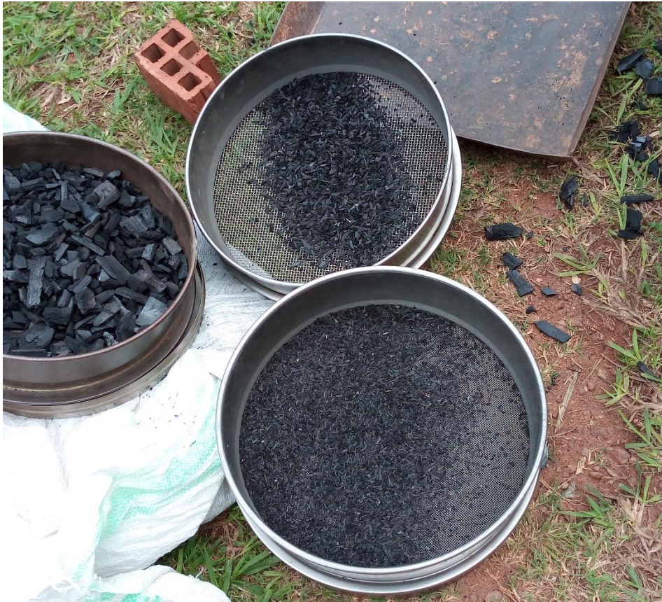
Figure 12-Sieve analysis of bamboo charcoal
