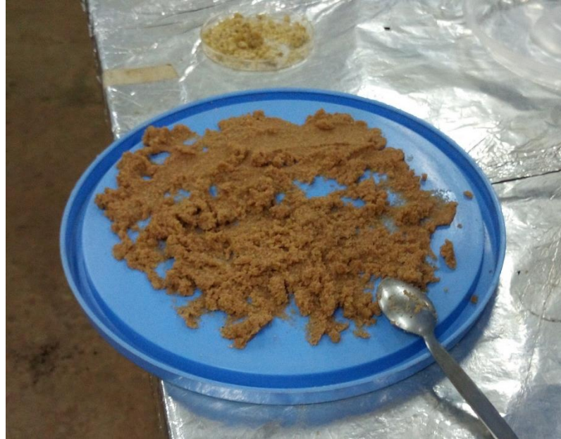
Figure 14- Prepared Functionalized sand
