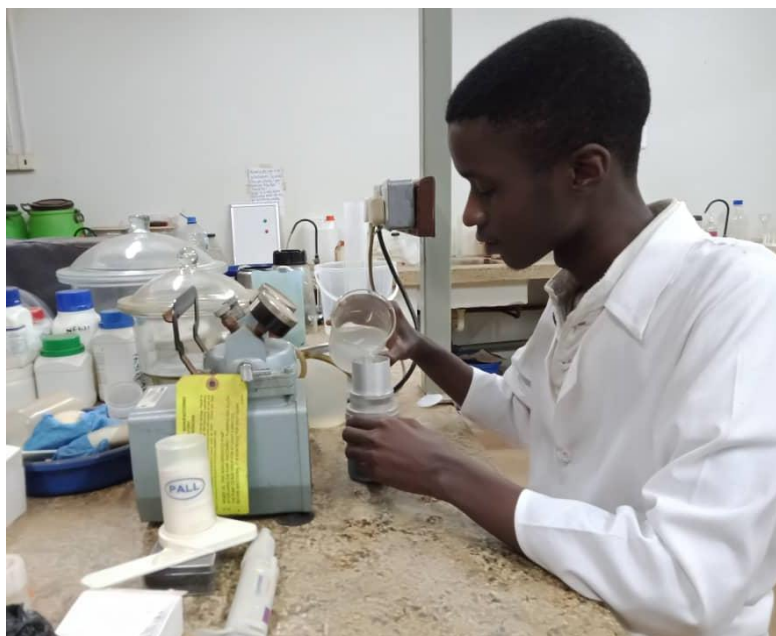
Figure 2: Filtration of the solution through the 2.5 \mu m
